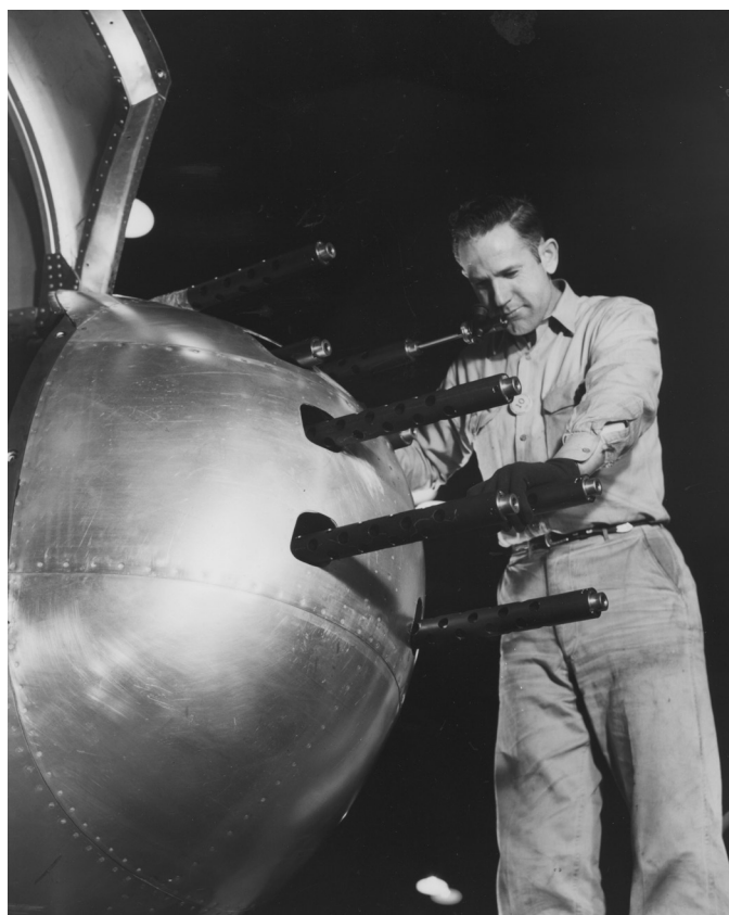
An armament worker reviews the completed installation of the eight .50 caliber machine guns in the nose of a J model B-25. The new model featured more machine-gun armament than the D model, outfitted with a total of either twelve or eighteen .50—caliber machine guns, thus providing a more lethal weight of attack. Courtesy of the Wyandotte County Museum.
