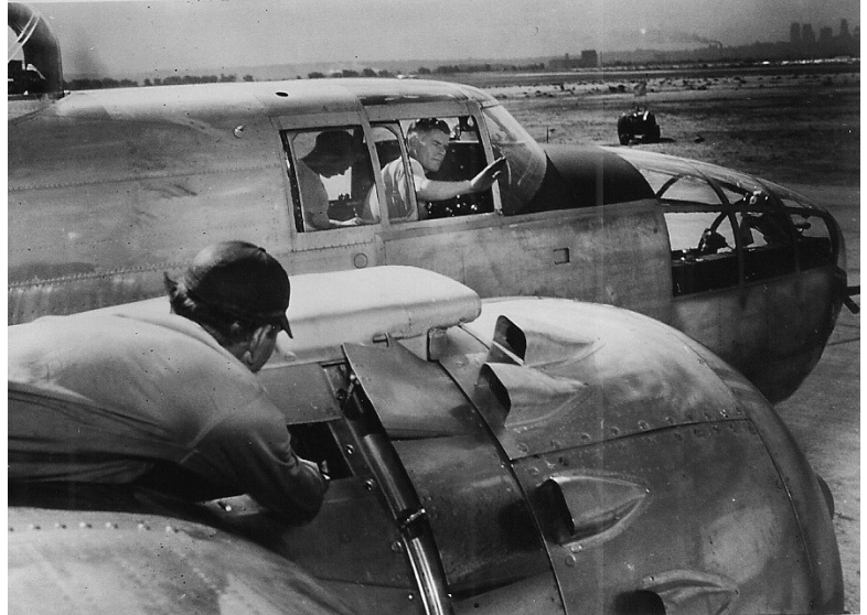
All newly-completed airplanes underwent rigorous pre-flight testing, with a crew chief and three or four mechanics in charge of this crucial procedure. In this photograph, crew chief Elmer Brown, sitting in the co-pilot's seat, signals to his mechanic atop the wing, while the mechanic makes an engine adjustment. Courtesy of the Wyandotte County Museum.
