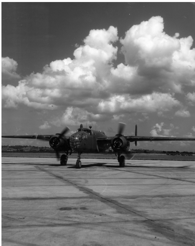
A test crew is performing an engine run-up on a flight line ramp. After ensuring that all pressures, temperatures, and speeds are within tolerance, the crew will move this B-25D into position on a runway for takeoff. Courtesy of the Wyandotte County Museum.
