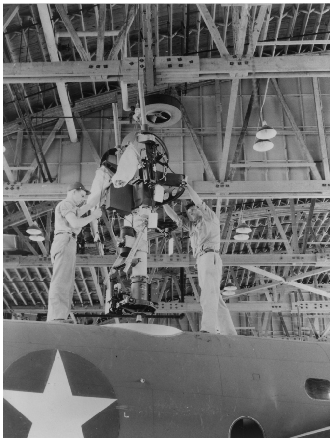
The B-25D had two turrets, one on the bottom and one on the top, the latter being installed in the photo above. Faced with an accelerated production schedule and the loss of men to military service, the NAA in 1943 changed its employment entry requirements, with one result being an increase in the number of female workers. Though only men are shown here, 39 percent of NAA's Kansas division was women by the fall of 1943. Courtesy of the Wyandotte County Museum.
