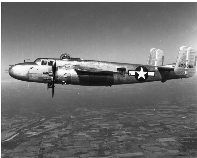
NAA and AAF test pilots, along with the crew chief—serving as co-pilot—meticulously checked the plane's functionality and performance. If all was satisfactory, they signed a Final Acceptance Form 262 signifying that the government had officially "bought" the airplane. Pictured here is a B-25J with eight-gun nose during a flight test. Courtesy of the Wyandotte County Museum.
